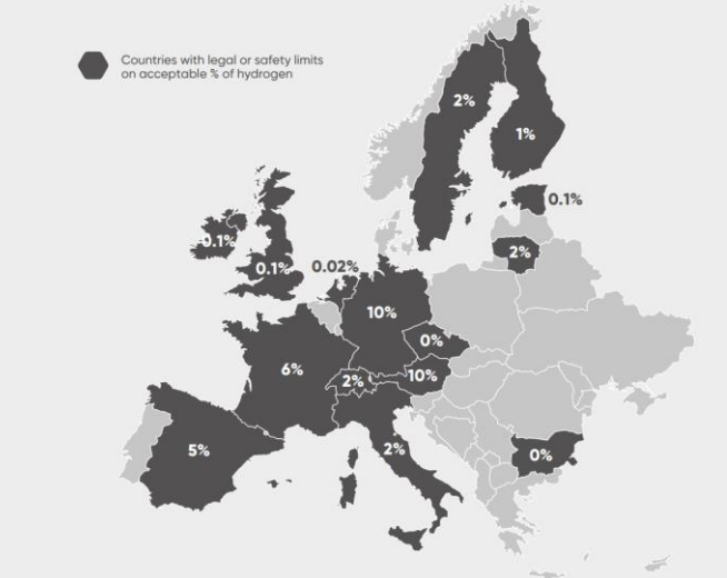
FIGURE 4 Maximum admitted percentage of hydrogen (by volume) in various European countries' transmission networks
