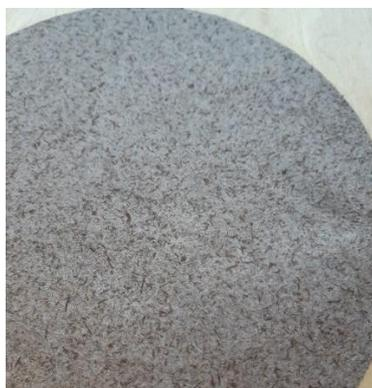
Figure 3. Fungal hyphae and cellulosic fibre composite material KF FF 50/50
