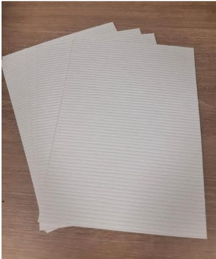
Figure 1. Kraft fibre sheets
