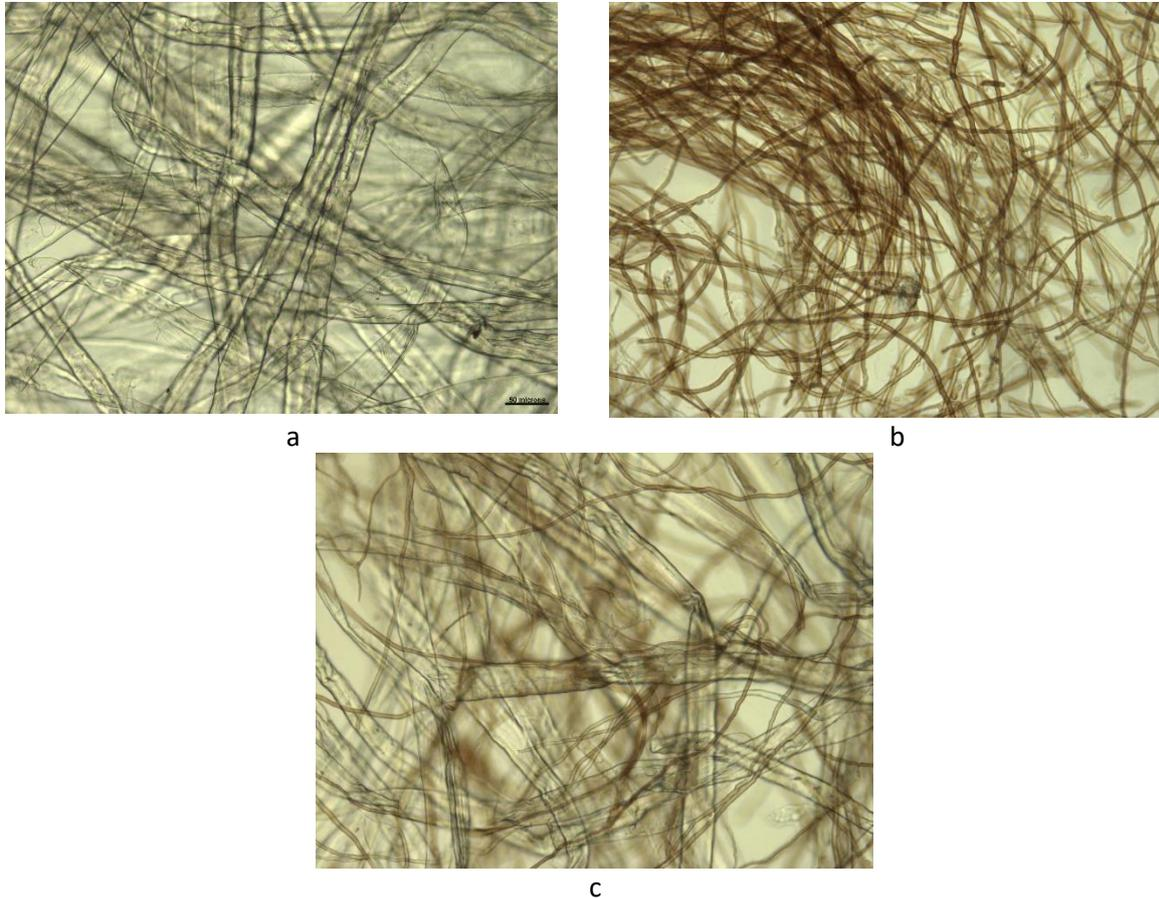
Figure 5. KF fibres 30  $\mu\text{m}$  in diameter (a), fungal fibres (hyphae) 3-6  $\mu\text{m}$  in diameter (b) and composite material KF FF 50/50 (c); LM 200x
