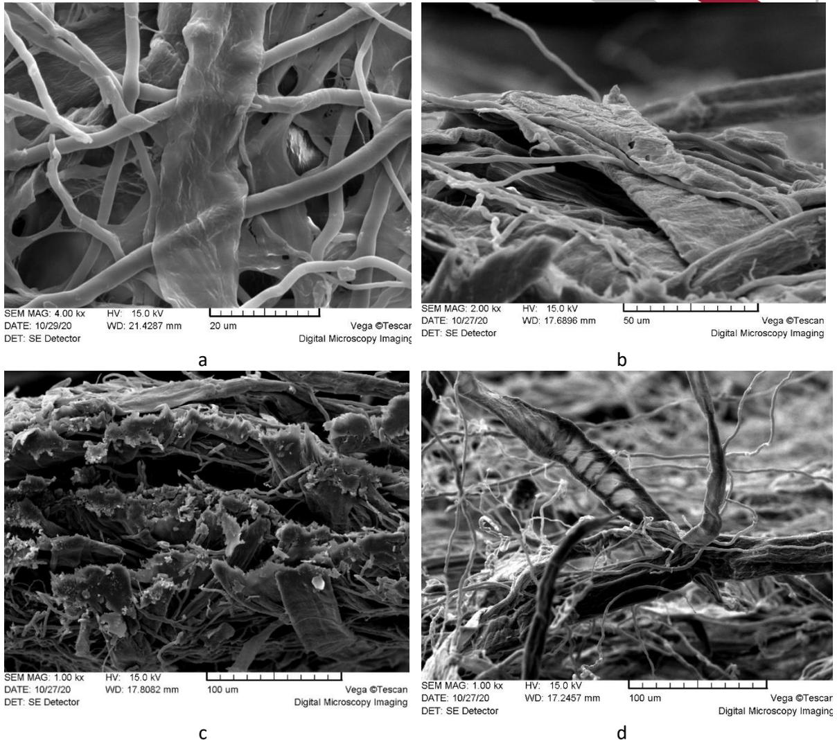
Figure 6. SEM microscopy of fungal hyphae and cellulosic fibre composite material membrane: a,b surface structure; c – cross section, cut; cross section, torn.
