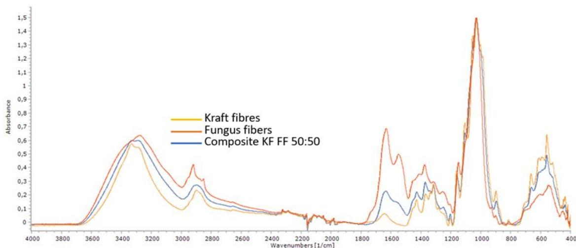
Figure 7. FTIR spectra of raw materials and composite material.
