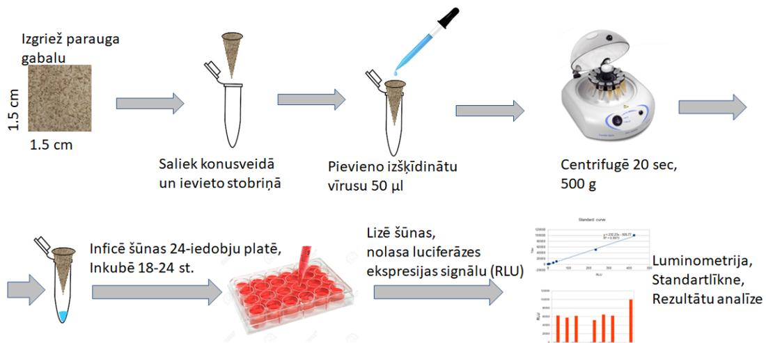
Figure 6. Schematic representation of the virus pressure filtration test.
