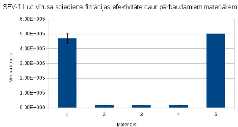
Figure 7. SFV1 / Luc virus pressure filtration efficiency through test materials. 1 - surgical mask; 2-cellulose fiber material; 3. cellulose and mushroom fiber composite material; 4. basidium mushroom fiber material; 5. control SFV-1 Luc virus  $5 \times 10^5$  iu, without filtration.
